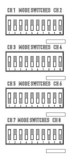
"MODE" configuration DIP switches are located on the rear panel and look like the illustration above. Switch positions shown are for example only. Set switches as required for your application.
